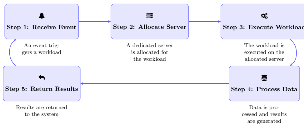
Figure 1: Serverless architecture cycle.
