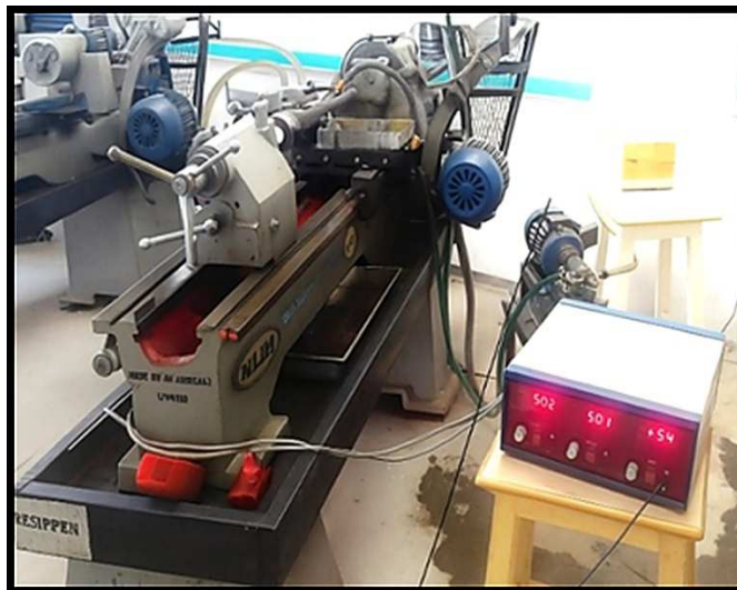
Fig. 1 Lathe Tool Arrangement with Measurement Instruments
