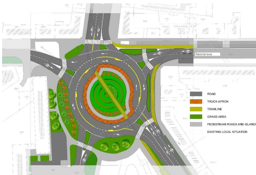
Figure 4 Fitting the designed turbo roundabout into the existing environment [10]
