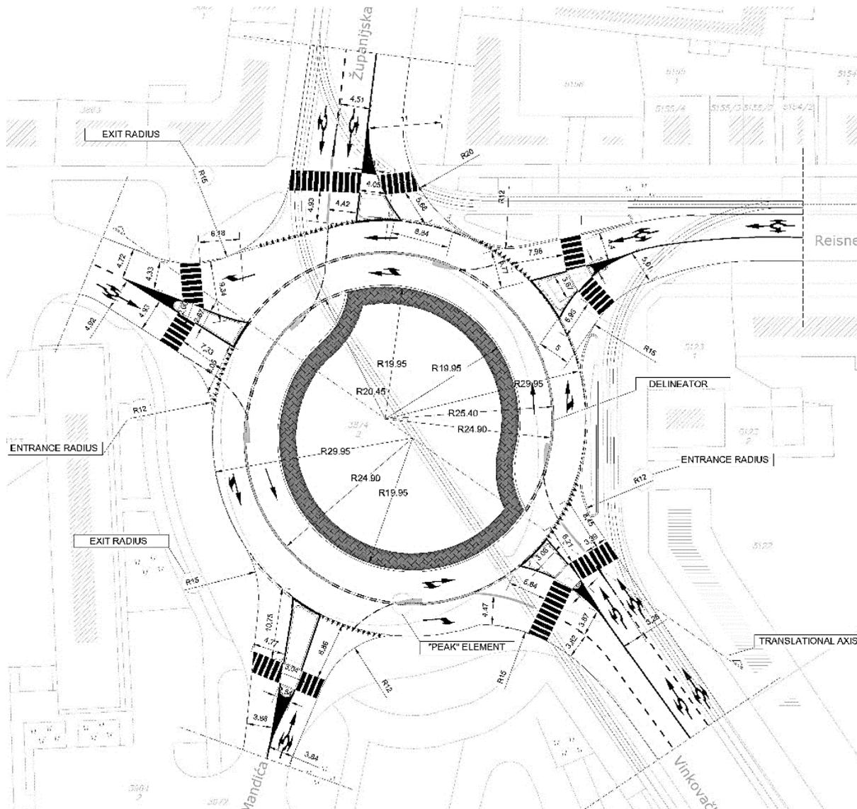
**Figure 3 Conceptual design of the turbo roundabout [10]**
