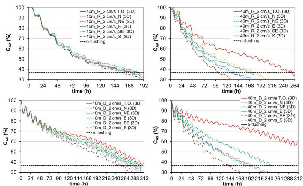
**Figure 8** Dynamics of the mean tracer solution concentration in the marina basin during the simulation period at the locations Rovinj (up) and Dubrovnik (down), for the marina entrance widths of 10 (left) and 40 m (right) (outer sea current speed of 2 cm/s,  $L/B=2$ ) for the case of tidal oscillations (T.O.) and wind from N, NE, E, SE and S direction (all for 3D model)
