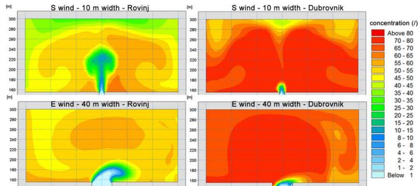
**Figure 5 Vertically averaged concentration field fields (3D model) for the 96th hour of numerical simulation at 2 cm/s currents outside the marina, for the E wind and the marina entrance width of 40 m, and for the S wind and entrance width of 10 m, locations Rovinj and Dubrovnik ( $L/B = 2$ )**
