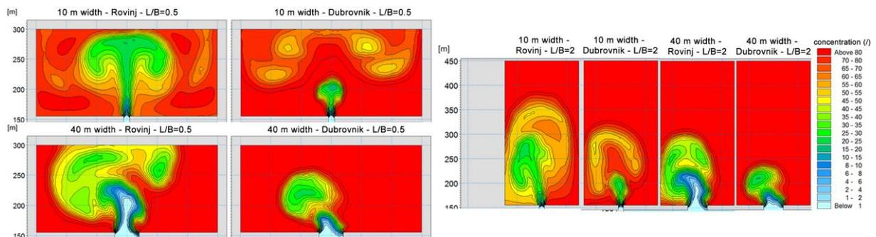
**Figure 4.** Vertically averaged concentration fields (2D model) for the 48th hour of numerical simulation at 2 cm/s sea currents outside the marina, marina entrance widths of 10 and 40 m, and for Rovinj and Dubrovnik locations ( $L/B = 2$  and  $L/B = 0.5$ )
