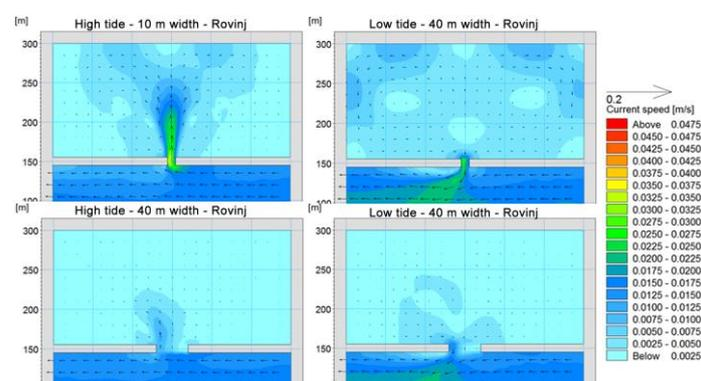
**Figure 2** Vertically averaged current velocity fields (2D model) for the 21st hour (low tide) and 28th hour (high tide) of the numerical simulations for 2 cm/s sea currents outside the marina, the marina entrance width of 10 and 40 m, location Rovinj, ( $L/B = 2$ )
