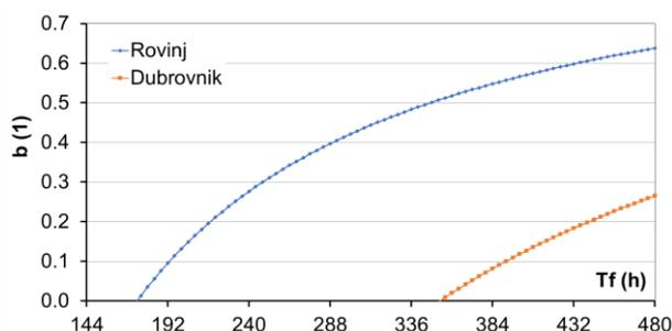
**Figure 9** Values of return flow factor  $b$  in relation to  $T_f$  (half day tidal period – 12.42 h  $V_{P0-SR (ROVINJ)} = 17703$  m<sup>3</sup>;  $V_{P0-SR (DUBROVNIK)} = 8713$  m<sup>3</sup>)
