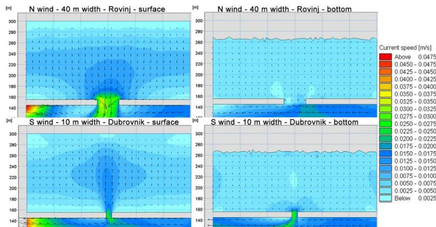
**Figure 3** Surface and bottom current velocity fields (3D model) for the 28th hour of numerical simulation at 2 cm/s sea currents outside the marina, for the marina entrance width of 10 m, at the location Dubrovnik and the S wind and for the marina entrance width of 40 m, location Rovinj and N wind (both  $L/B=2$ )
