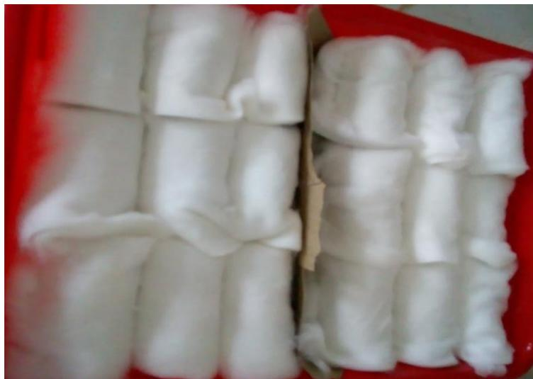
Figure 2 Specimens Subjected to Wetting Cycle for 24 hours
