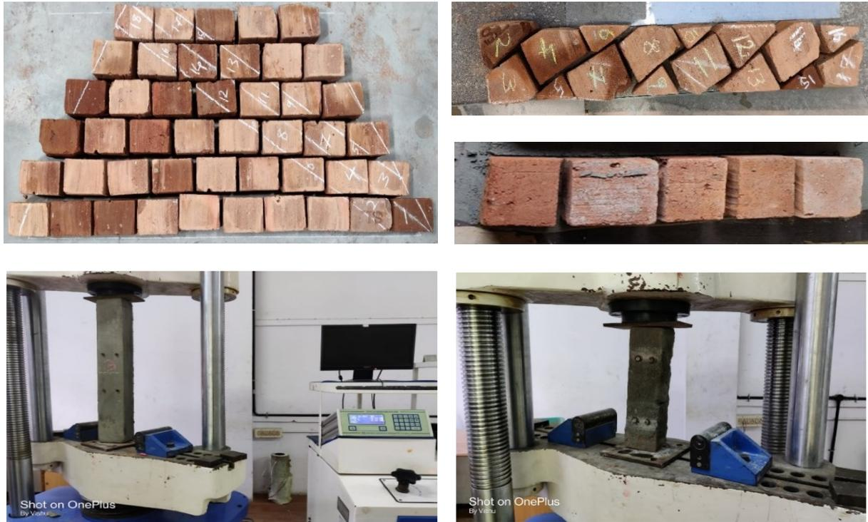
**Figure 10. Test of normal and inclined bed joints**
