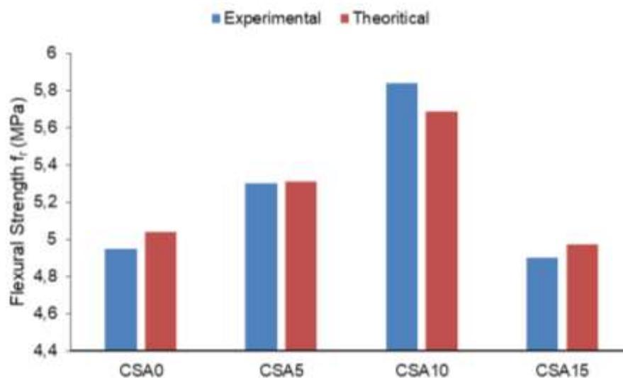
Figure 10. Experimental and theoretical flexural strength of alccofine supplemented CS concrete
