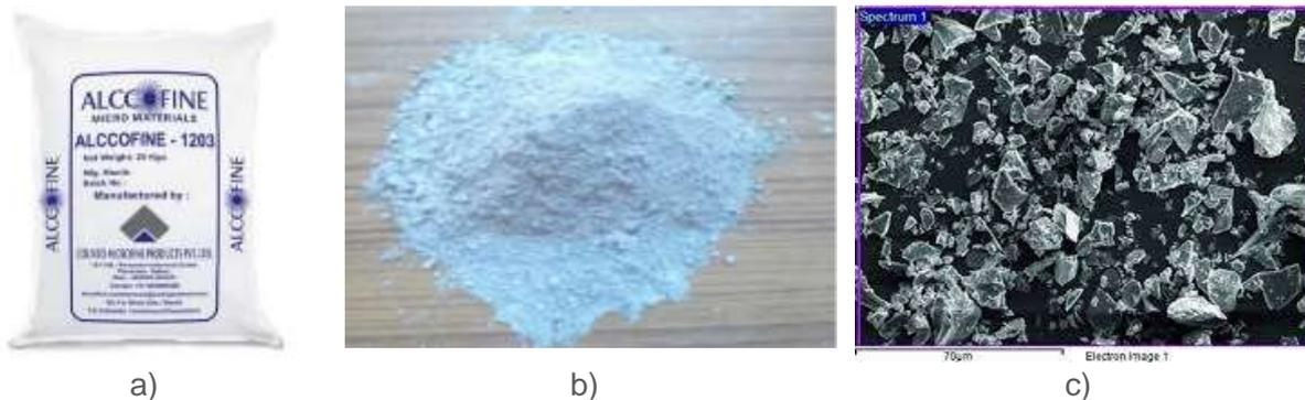
Figure 1. a) Alccofine pack, b) Alccofine sample, c) SEM image
