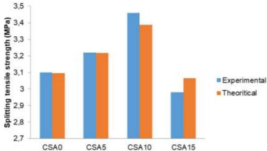
**Figure 8. Experimental and theoretical split tensile strength of alccofine supplemented CS concrete**
