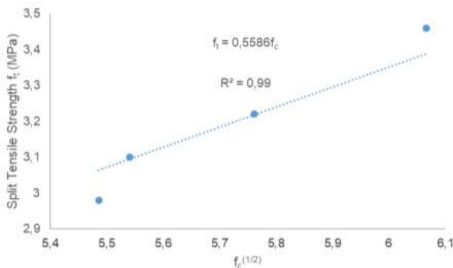
**Figure 7. Correlation between compressive strength and split tensile strength of alccofine supplemented CS concrete**
