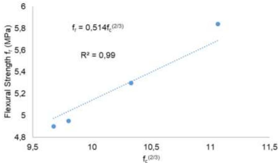
Figure 9. Correlation between compressive strength and flexural strength of alccofine supplemented CS concrete
