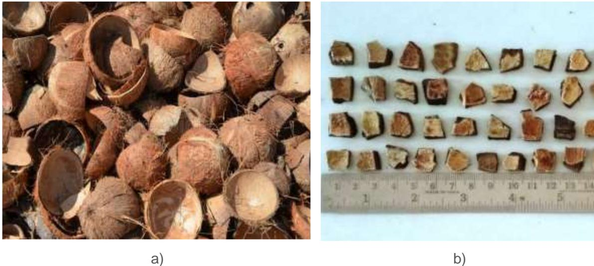
**Figure 2. a) Discarded CS waste from copra preparation yard, b) Aggregates crushed from CS shell**
