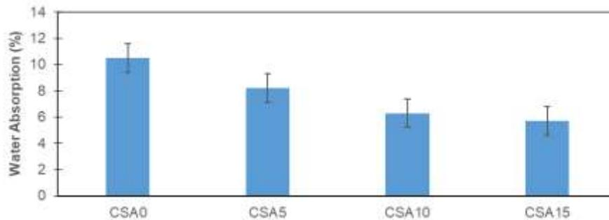
Figure 11. Water absorption of alccofine supplemented CS concrete
