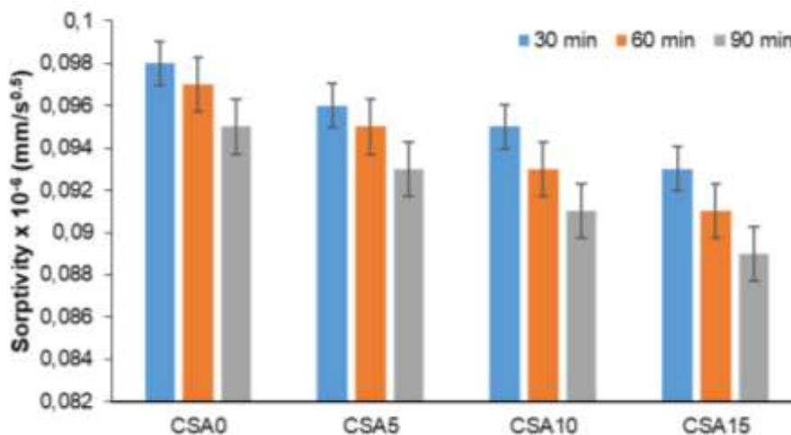
Figure 12. Sorptivity of alccofine supplemented CS concrete
