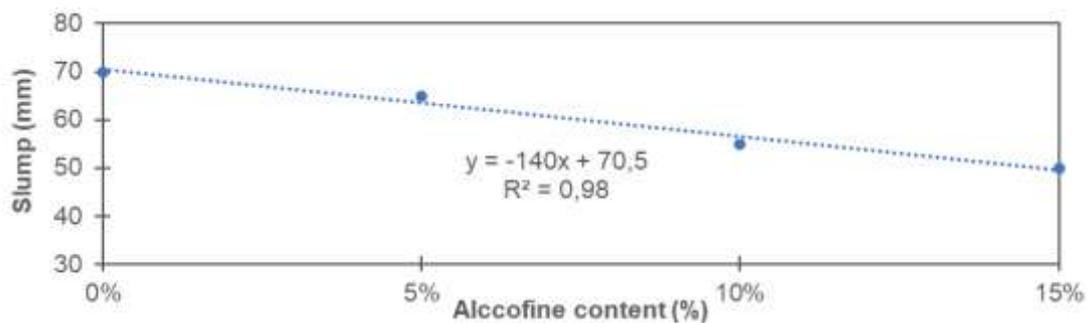
Figure 4. Influence of Alccofine content on slump of CS concrete
