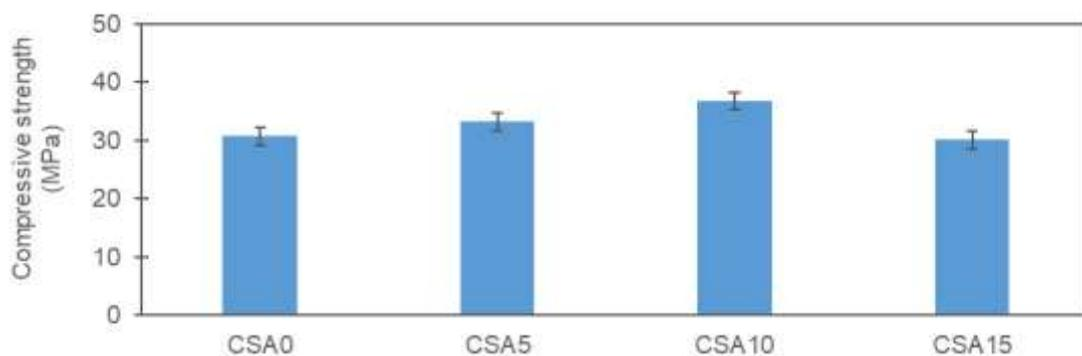
Figure 6. Compressive strength alccofine supplemented CS concrete
