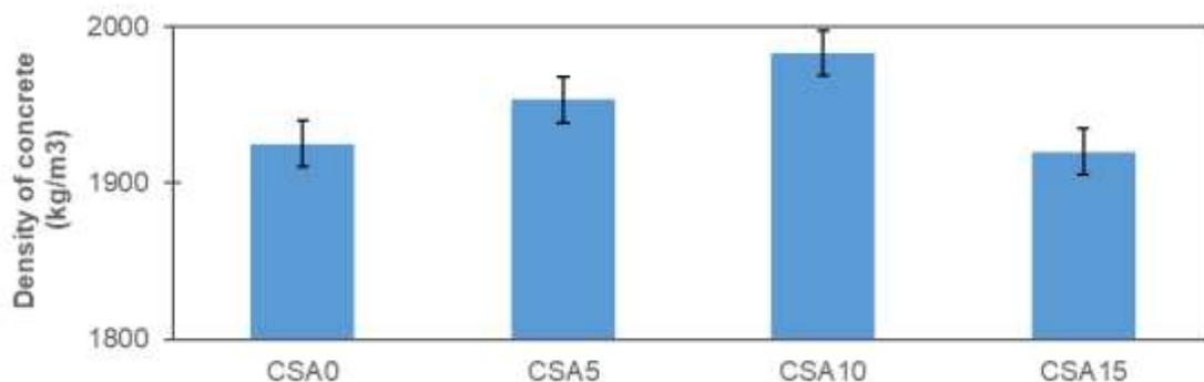
Figure 5. Influence of alccofine content on density of CS concrete
