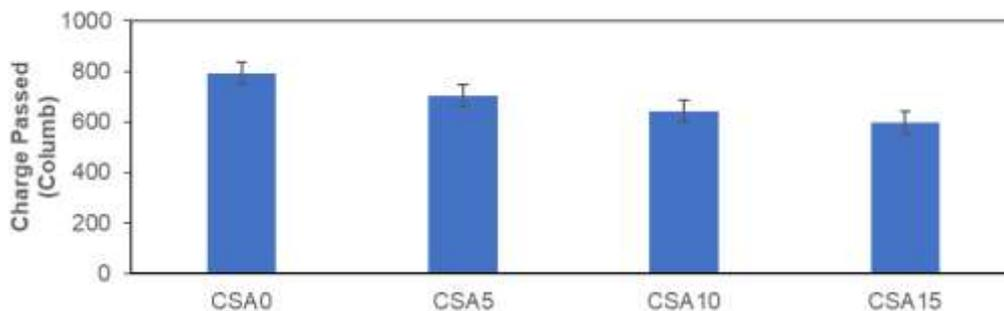
Figure 13. Charge passed of alccofine supplemented CS concrete
