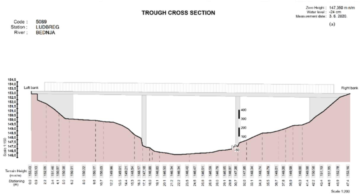
Figure 7. Cross-section profile of the Ludbreg measurement station on the Bednja River [34]
