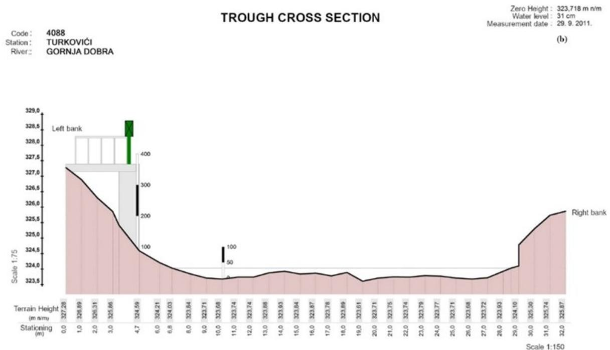
Figure 8. Cross-section profile of the Turkovići measurement station on the Gornja Dobra River [34]
