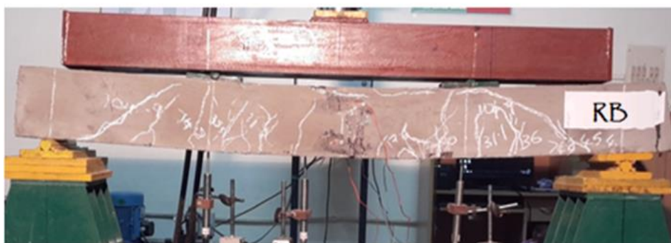
Figure 8. Crack pattern of the grouted pre-damaged beam
