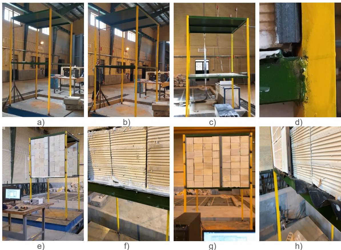
Figure 5. Representation of five types of 3D two-story frame structures: (a) Type I, (b) Type II, (c) Type III, (d) wall post-frame connection, (e) Type IV, (f) Type IV wall-frame connection, (g) Type V, (h) Type V wall-frame connection
