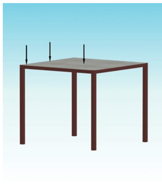
Figure 8. Schematic of the primary mass modelling approach for frames
