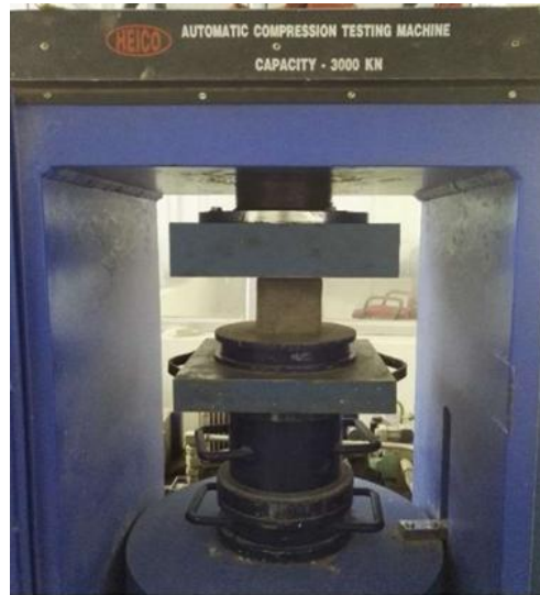
Figure 4. Compressive-strength test setup
