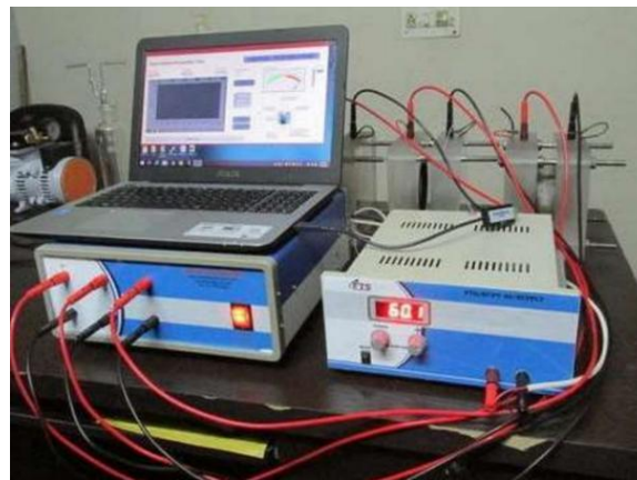
Figure 6. Rapid chloride permeability test in progress
