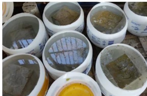
Figure 7. GC samples immersed in acidic solution
