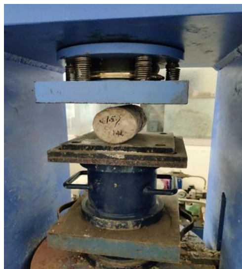
Figure 5. Setup for split-tensile-strength test
