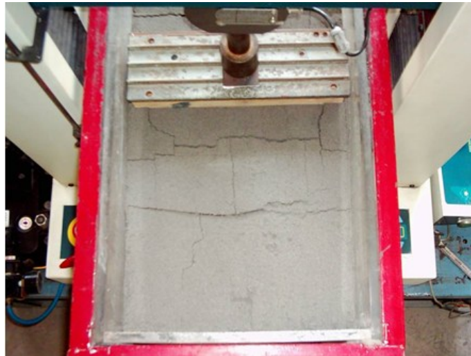
Figure 5. Top view of model tank at the end of loading
