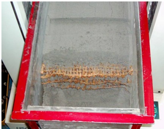
Figure 6. Coir geosynthetics reinforcement after completion of loading
