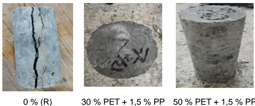
Figure 14. Mode failure of splitting tensile specimens
