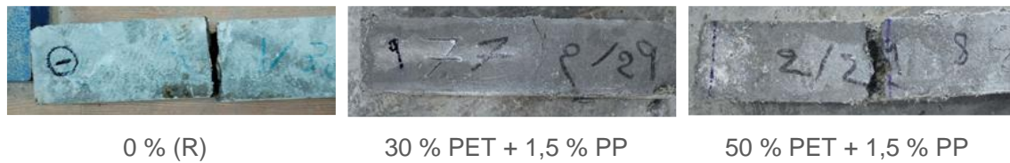
Figure 15. Mode failure of flexural specimens
