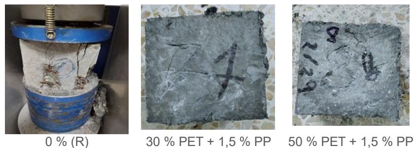
Figure 13. Mode failure of compressive specimens
