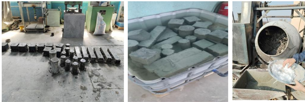
Figure 3. Process for pouring and curing concrete samples
