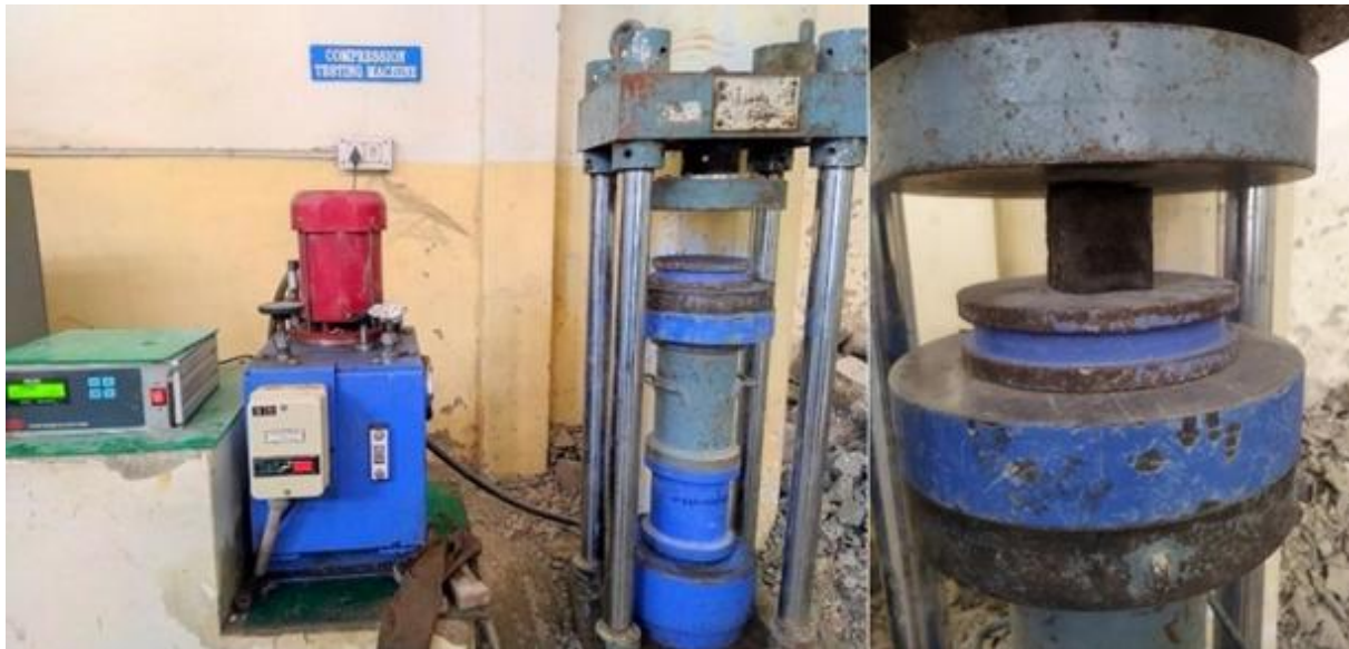
Figure 4. Compressive strength testing of geopolymer mortar specimens
