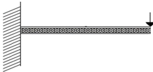
Figure 11. Clamped-free sandwich plate with a point load applied at the free end
