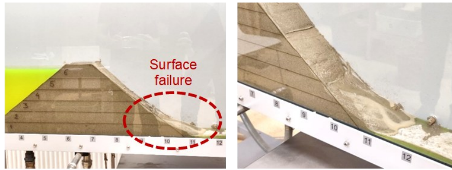
Figure 11. Sliding and failure of the downstream slope in Model 4
