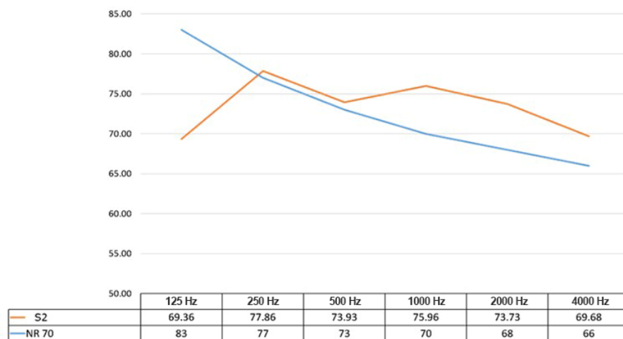
Figure 7. Interior noise levels of the industrial plant when it was covered with 100 % sound-absorbing materials
