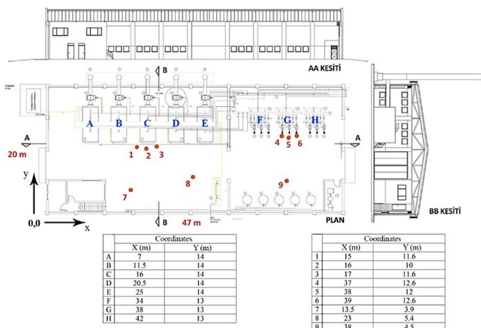
Figure 1. Plan of the industrial plant, machine layout, and measurement points
