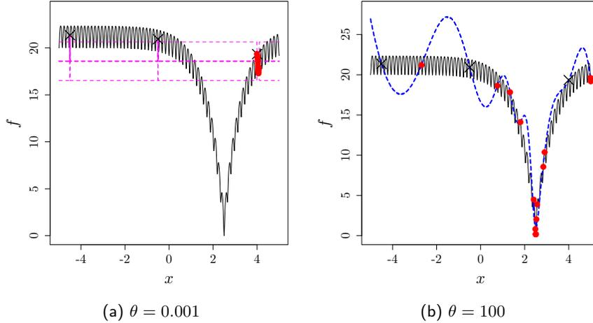
Figure 3: Ackley function (solid line) approximated by a kriging model (mean  $\pm$  std. deviation, thick/thin lines) with  $\theta = 0.001$  (dashed) and  $\theta = 100$  (dotted). The crosses are the initial DoE. Bullets: DoEs created by EGO after 20 iterations.
