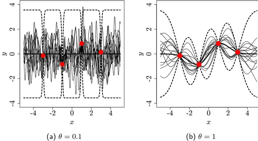
Figure 1: Kriging mean (thick solid line) along with the 95% confidence intervals (thick dashed lines), i.e.,  $m(\mathbf{x}) \pm 1.96s(\mathbf{x})$ . The thin lines are the sample paths of the GP. As  $\theta$  changes, the class of possible functions considered for the optimization decision changes.
