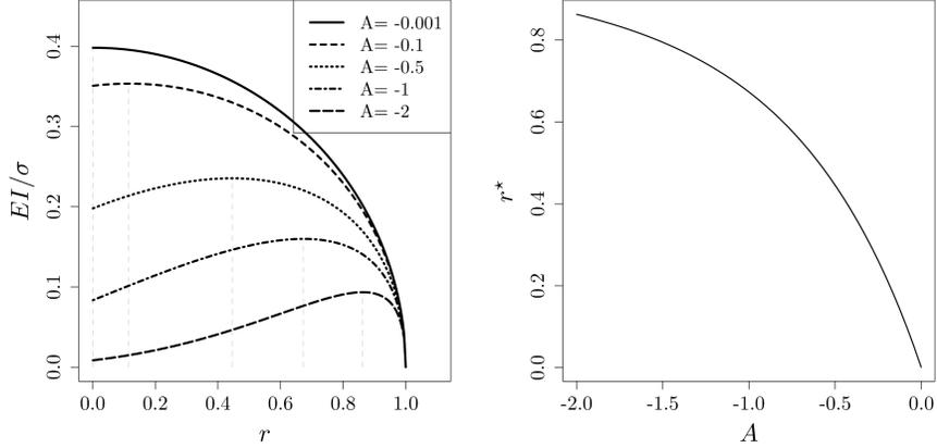
Figure 2: *Left: Normalized EI as a function of  $r \in [0, 1]$  in the vicinity of the sample point with the lowest function value for a small length scale. Right: location of the next EGO iterate ( $r^*$  where EI is maximized) as a function of  $A$ .*
