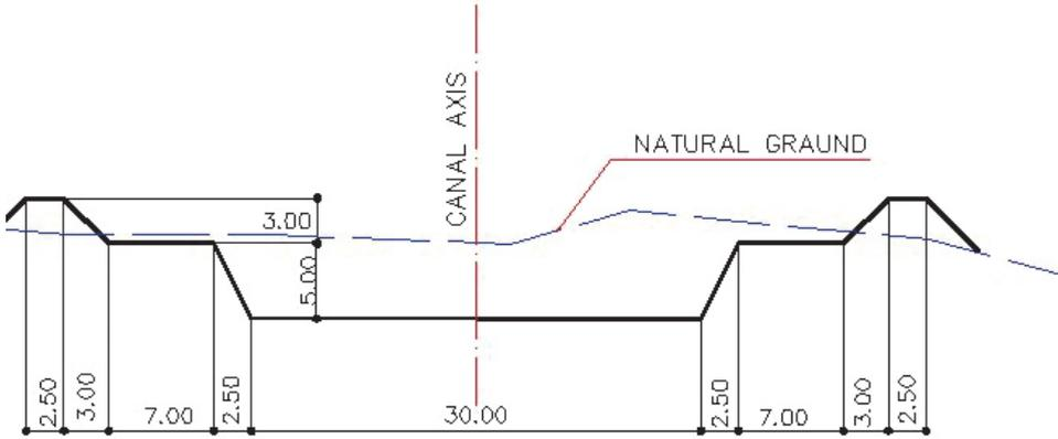
**Figure 11.** Canal typical cross section.
