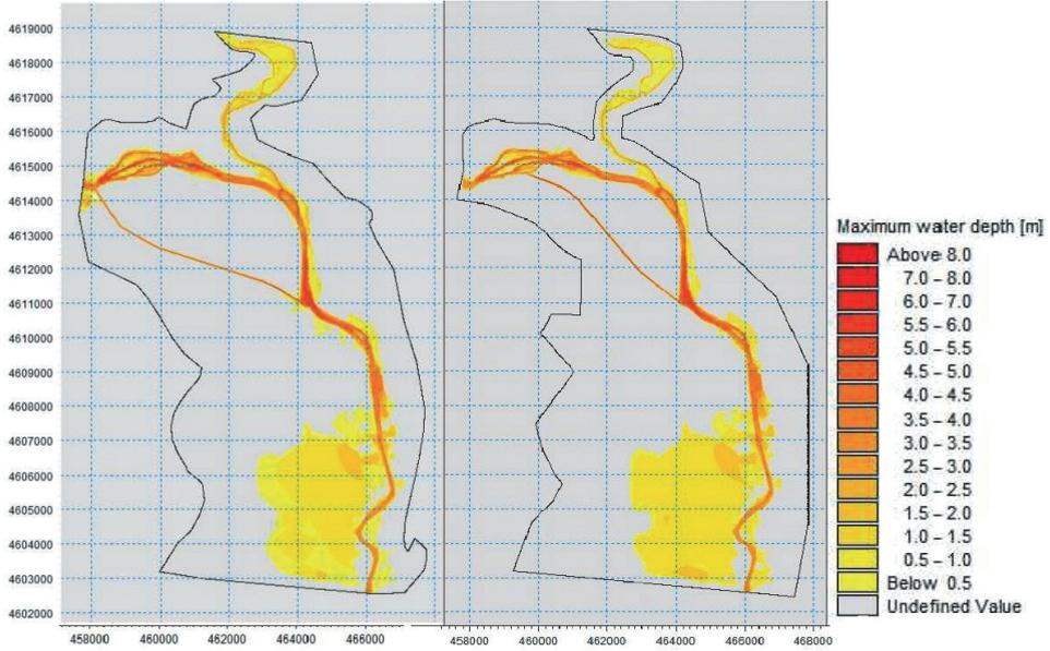
**Figure 14.** The 1<sup>st</sup> and the 2<sup>nd</sup> route 2D model downstream conditions.
