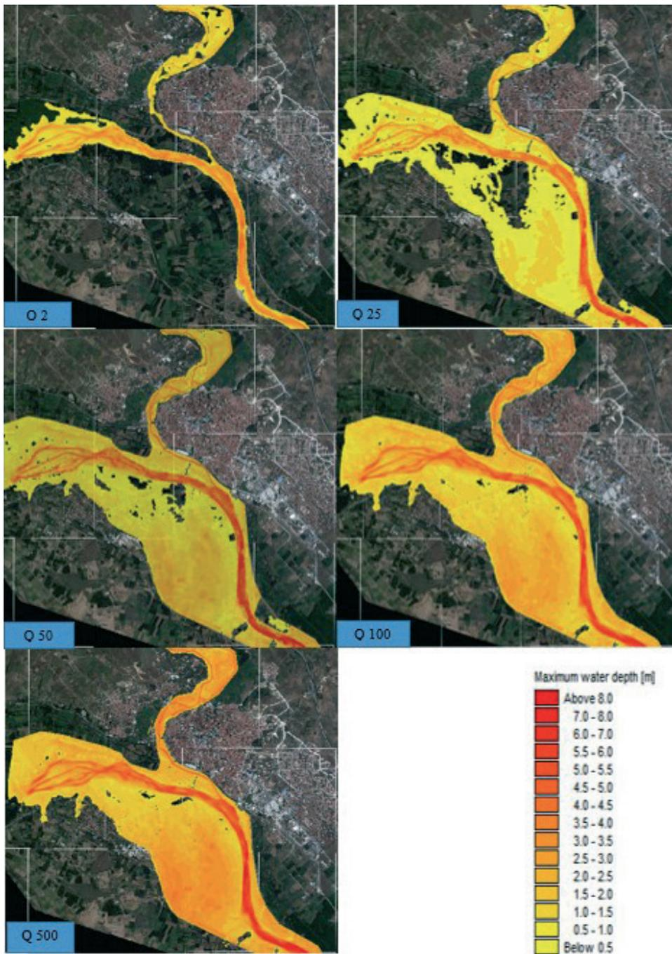
Figure 8. Q2, Q25, Q50, Q100, Q500 flood inundation maps.
