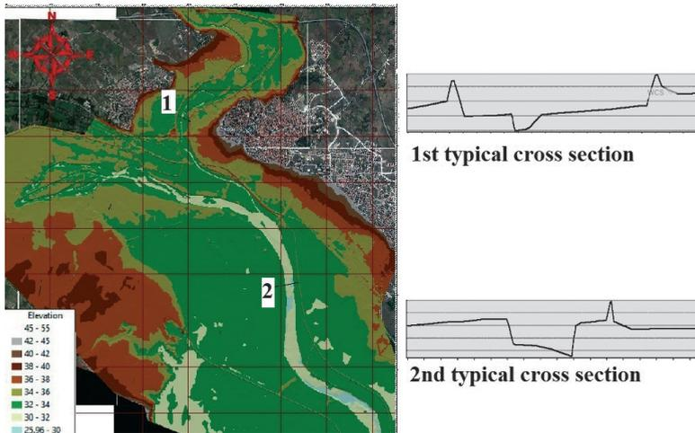
**Figure 4.** Study area topography and typical cross sections (*smaller figure*).
