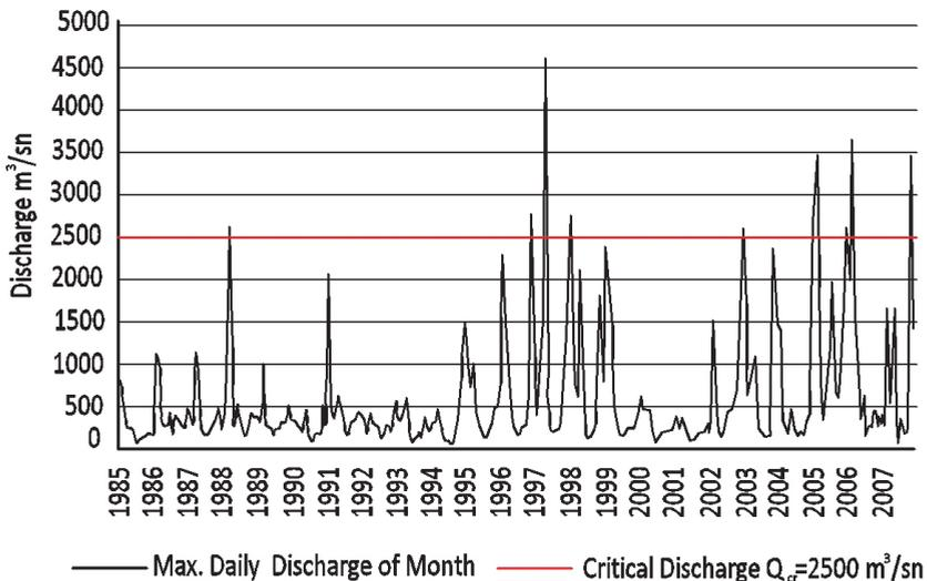
**Figure 3.** Maximum daily discharge rates of Meriç River from 1985 to 2007 (Angelidis et al., 2010).
