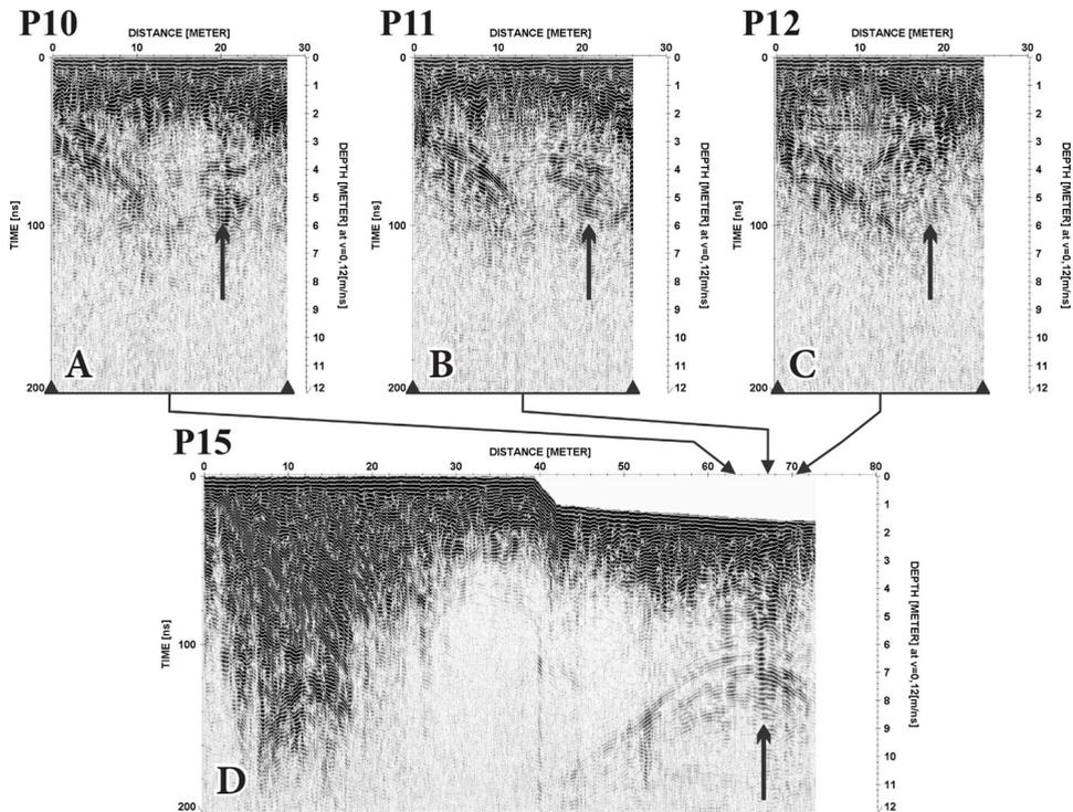
**Figure 3.** Selected radargrams received as a result of imaging with the use of shielded antenna 250 MHz showing the anomalous areas and forecasting occurrences of voids or loosening in rock mass transformed by the karst processes.
