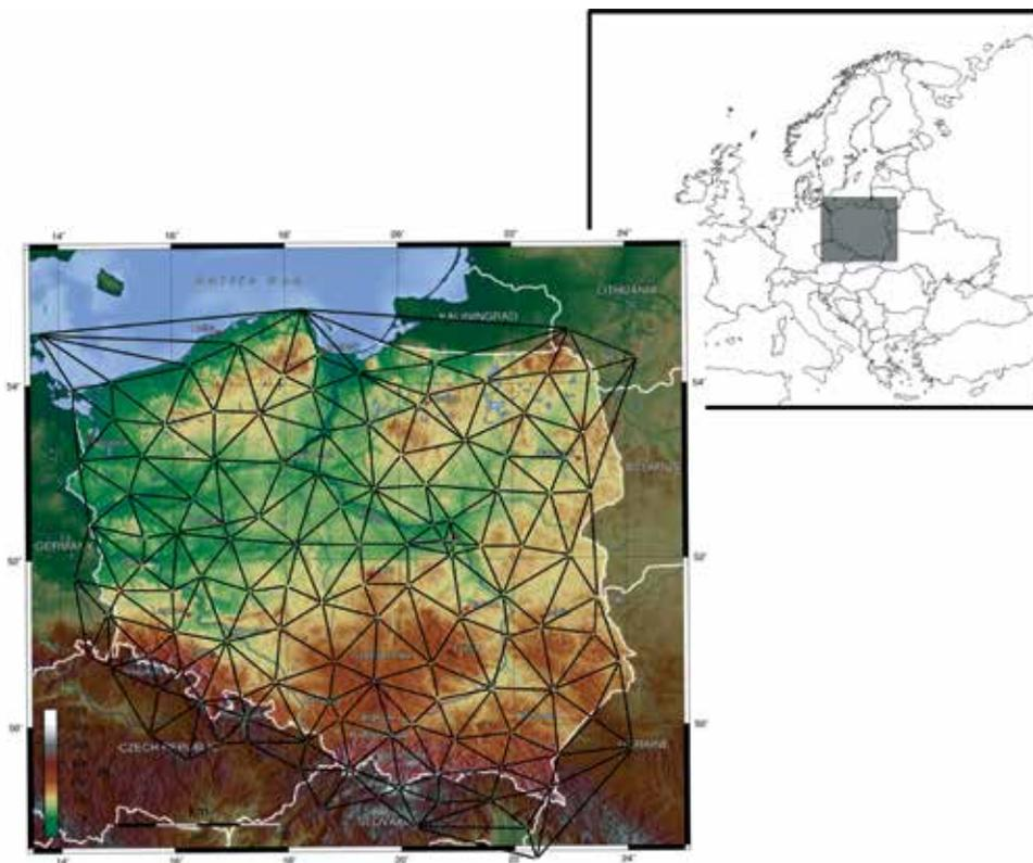
**Figure 1.** The baselines between the GNSS stations selected for the analysis (Central Europe) (topographic map © worldmap.pl by Webrange).
