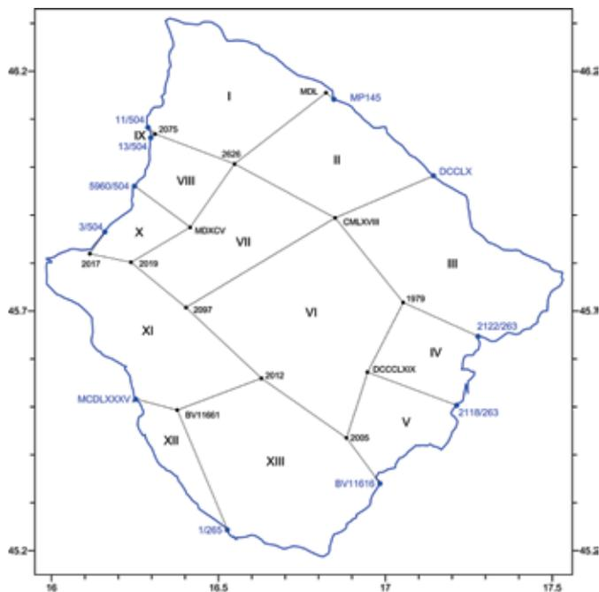
Figure 7. Scheme of II order levelling network geometrical configuration – loop no. III.
