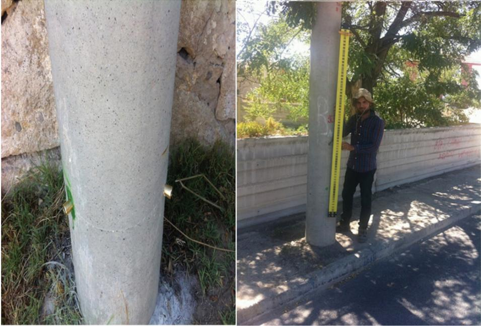
**Figure 3.** Blue and green benchmarks on the electrical pole.
