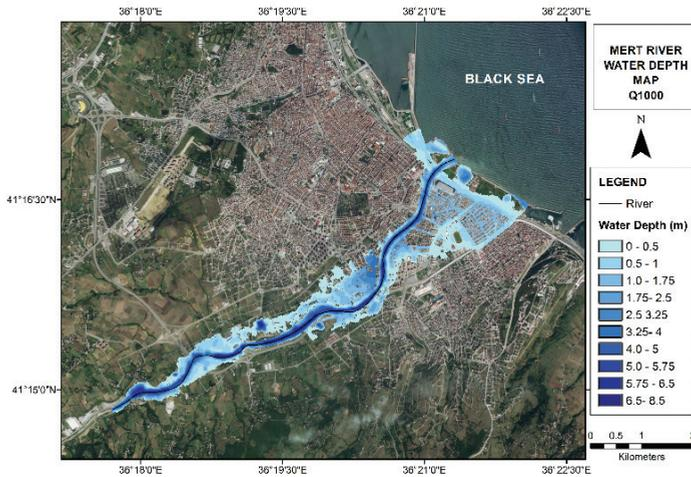
**Figure 13.** Water depth thematic map for a Mert River Q1000 discharge.
