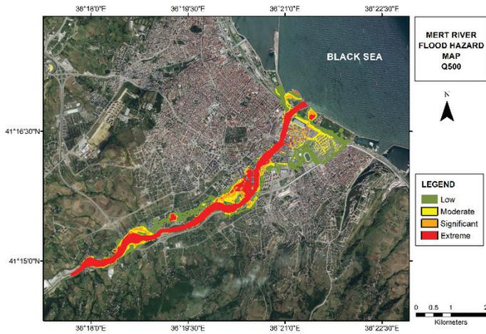
Figure 15. Flood hazard thematic map for the Mert River for a Q500 discharge.
