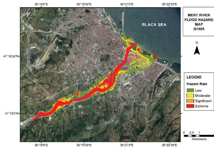
Figure 16. Flood hazard thematic map for the Mert River for a Q1000 discharge.
