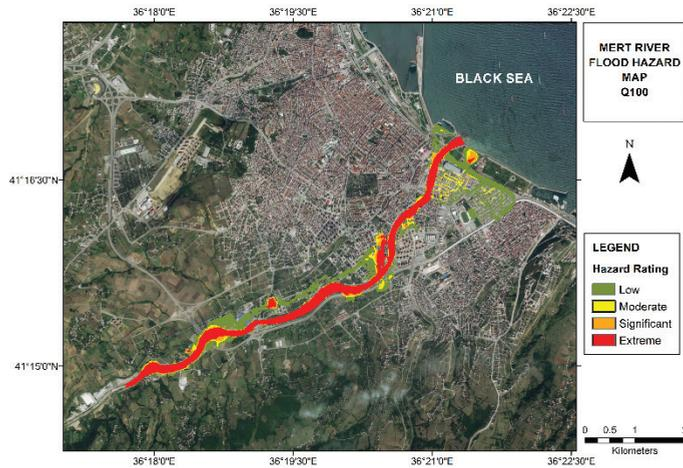
Figure 14. Flood hazard thematic map for the Mert River for a Q100 discharge.
