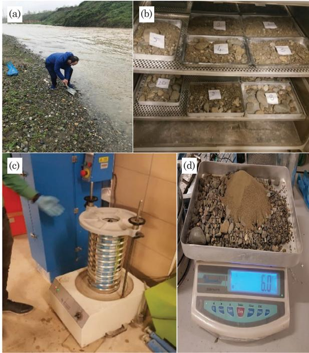
**Figure 3.** Sample sampling area (a), drying of samples in the oven (b), sieve shaking table (c), weighing the screened samples (d).
