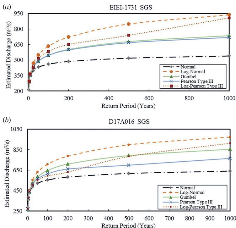
**Figure 3.** Discharge estimates with respect to probability distribution functions for different return periods: (a) SGS EIEI-1731, (b) SGS D17A016.
