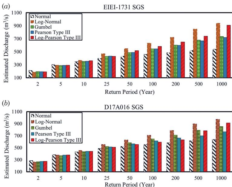
**Figure 4.** Comparison of flood frequency analysis results for stream gauging stations: (a) SGS EIEI-1731, (b) SGS D17A016.
