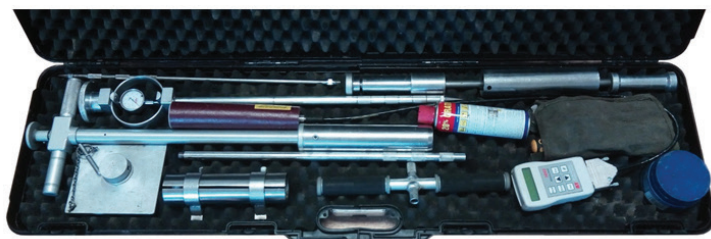
Figure 1. The original E-960 Soil Trafficability Kit, including attachments designed by the research team for easier handling and the ThetaProbe ML3 portable soil moisture sensor.
