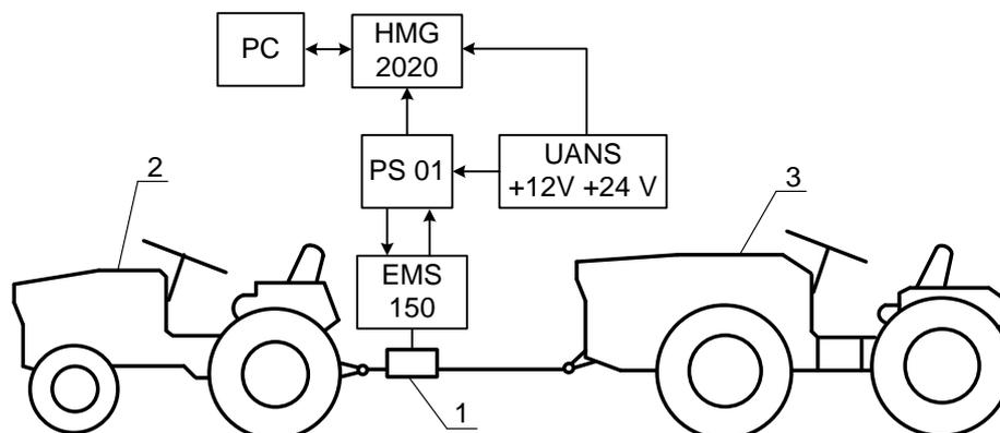
Figure 5: Connection diagram of drawbar pull measurement of Mini 070
