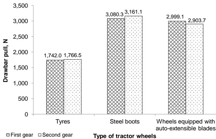
Figure 9: Maximum values of drawbar pull of Mini 070 on the grass
