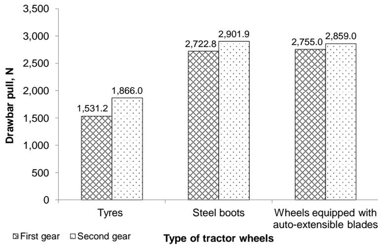
Figure 8: Maximum values of drawbar pull of Mini 070 on the soil
