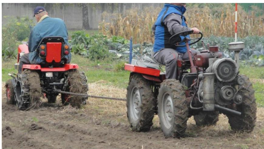
Figure 6: Measurement of drawbar pull
