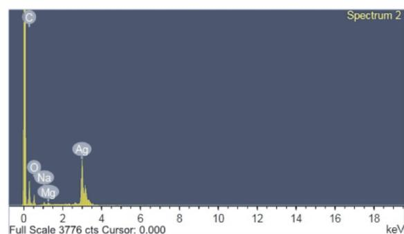
Figure 4. EDX pattern of Silver nanoparticles
