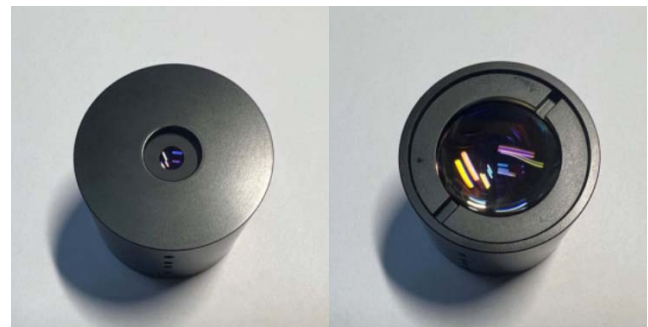
Figure 9 RLOS telecentric lens for UWOC. [22]
