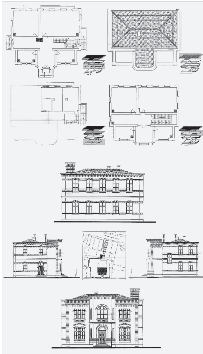
FIG. 10 YEDIKULE GERMAN SCHOOL RESTITUTION PLANS (UP) AND FAÇADES (DOWN) DRAWINGS
