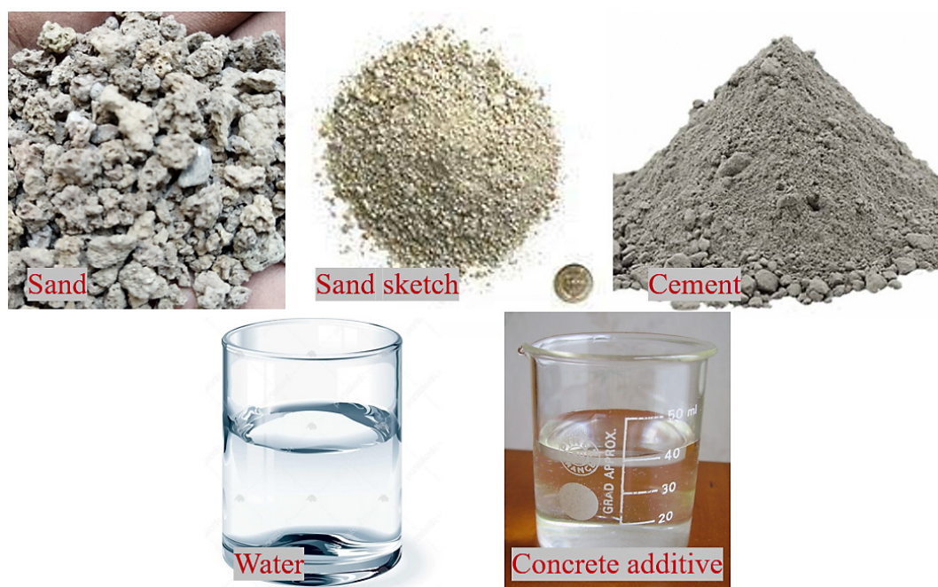
Figure 1: The materials used for preparing specimens i.e. sand, sand sketch, cement, water, concrete additive
