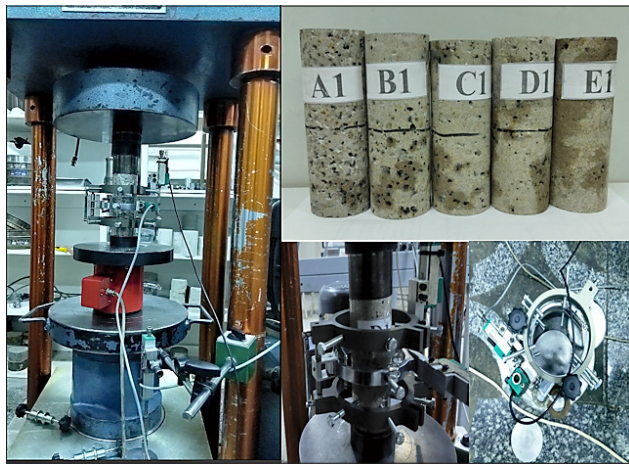
Figure 4: Uniaxial testing machine with displacement data logger and the prepared specimens
