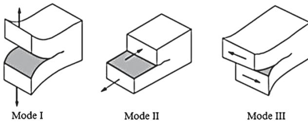
**Figure 1:** Schematic representation of various fracture modes (Erarslan and Williams, 2013)
