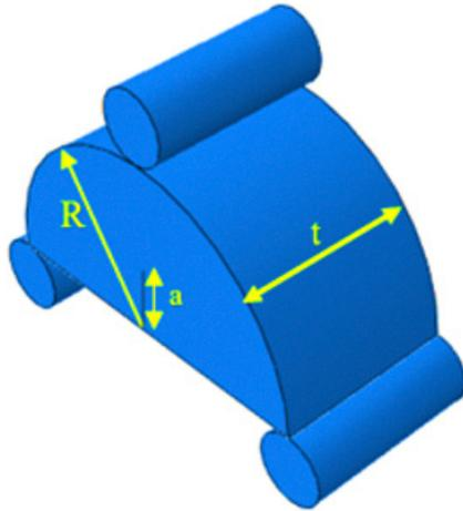
Figure 2: The semi-circular specimen under three-point bending (SCB)
