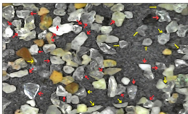
Figure 9: Broken sand fragments remain after the attrition process
