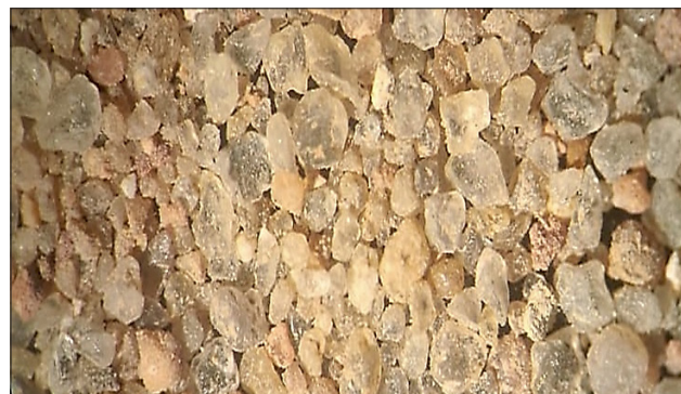
Figure 7: Classified sand sample showing an abundance of clayey coating on the grain surfaces
