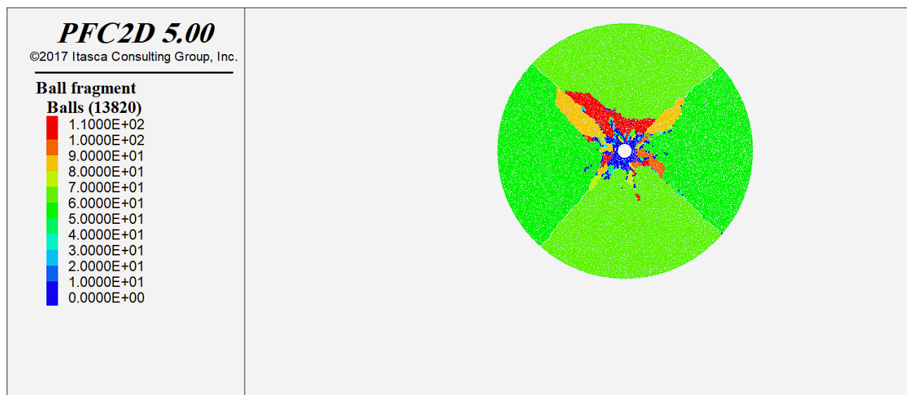
Figure 12: Distribution and size of the generated fragments during the simulation of shock and reflection energy
