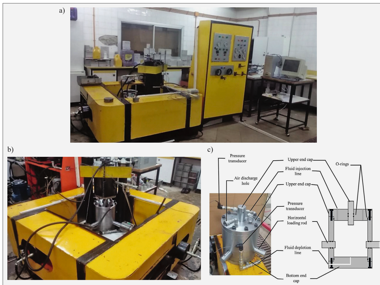
Figure 1: a) Overview of experimental setup; b) The frame and jack for applying axial pressure; c) Pore pressure cell developed to apply injection load on samples (Mortazavi and Atapour, 2018).
