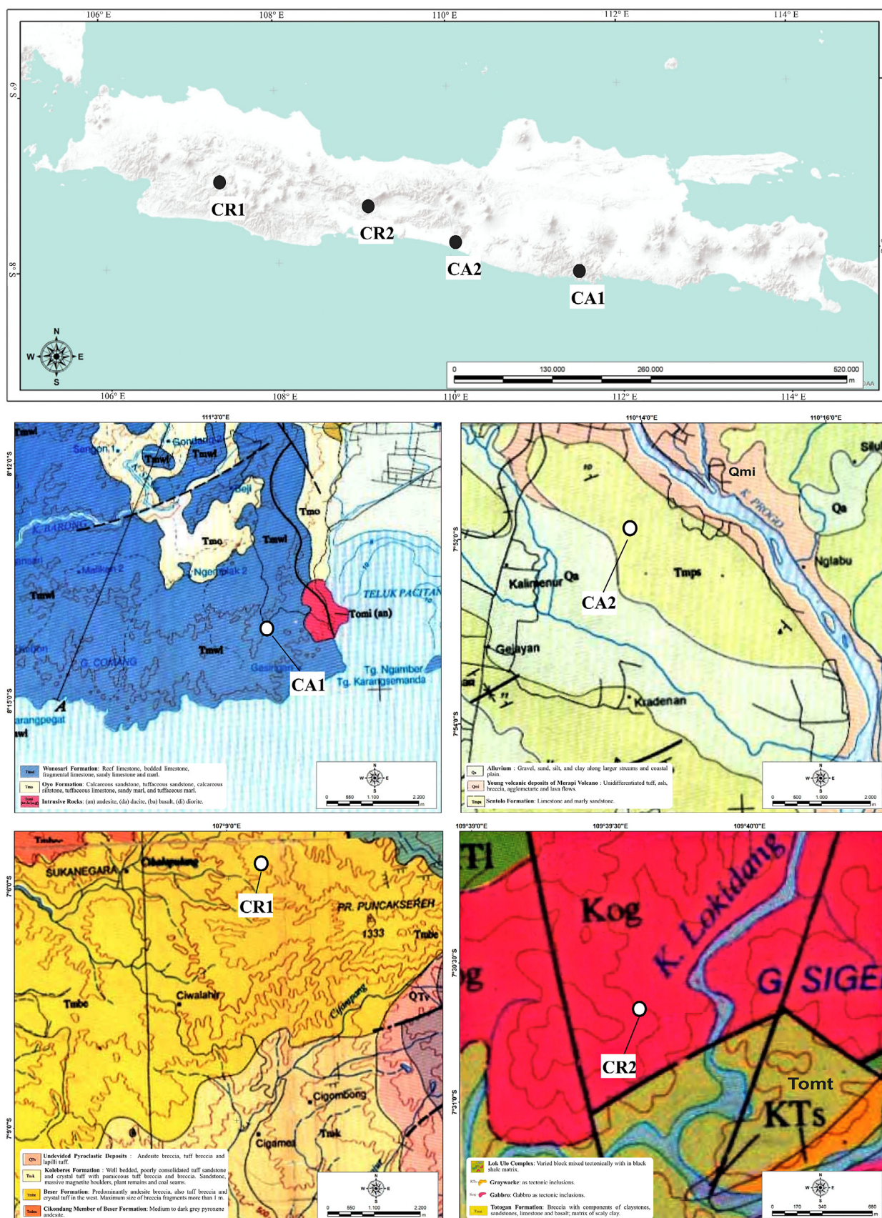
Figure 1. Drilling locations of rock samples from Java Island. CA1: Limestone from Wonosari Formation, East Java. CA2: Limestone from Sentolo Formation, Yogyakarta. CR1: Andesite from Beser Formation, West Java. CR2: Gabbro from Mount Parang, Central Java (modified from Samodra et al., 1992; Rahardjo et al., 1995; Koesmono et al., 1996; Asikin et al., 1992)
