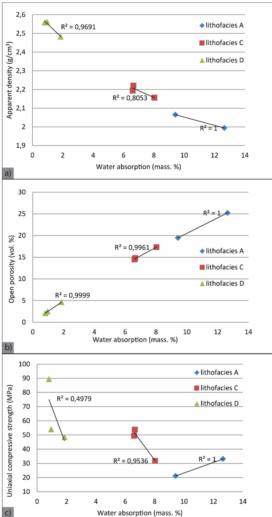
**Fig 13.** Diagrams for the correlation between: a) apparent density and water absorption b) open porosity and water absorption c) uniaxial compressive strength and water absorption, for samples from lithofacies A, C and D
