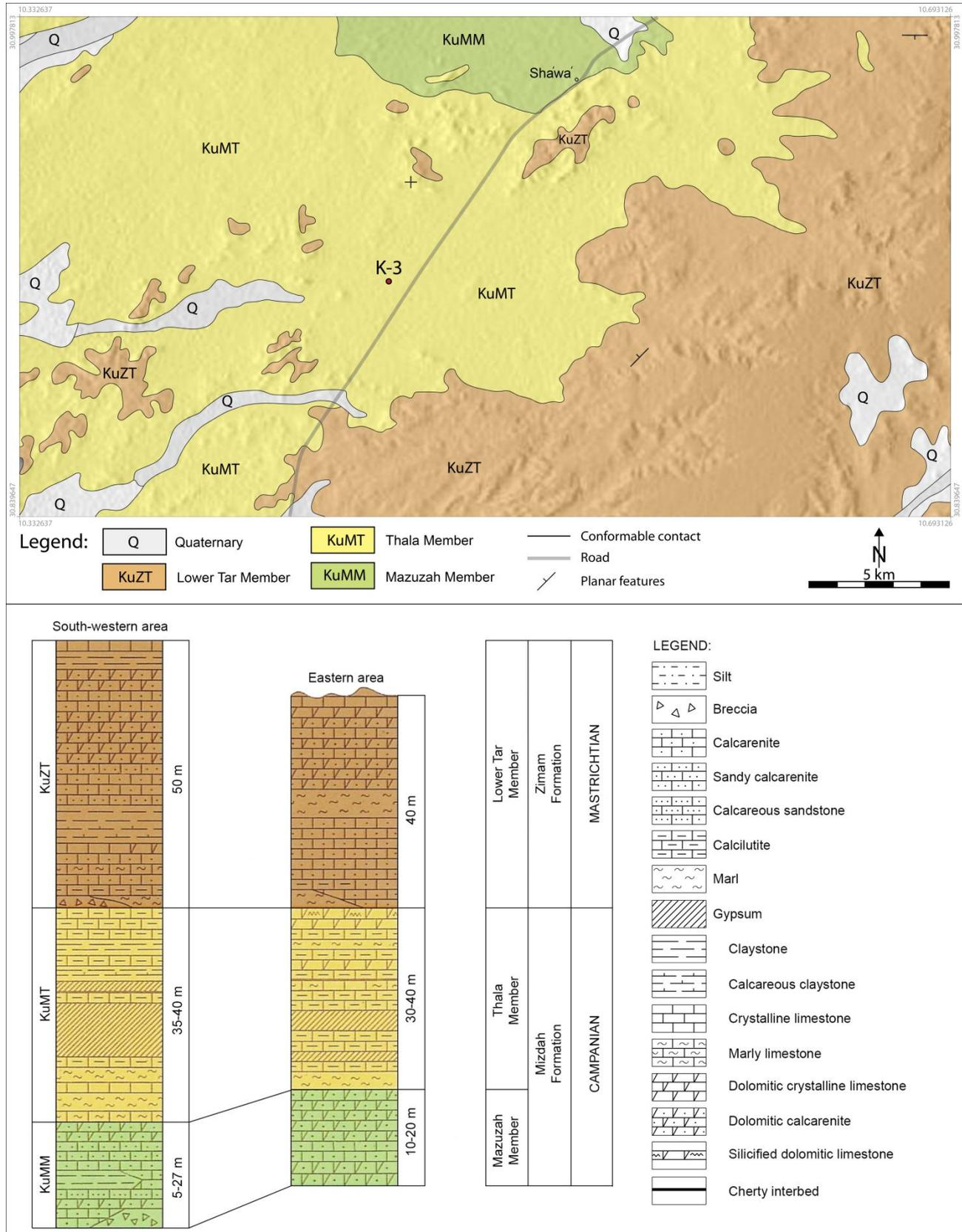
**Fig 3.** Geological map and the geological column of Sinawin- Sha'wa area (redrawn and adapted from Geological Map of Libya 1:250.000, Sheet Sha'wa – IRCT, 1979). Position of the K-3 Quarry site is marked on the map.
