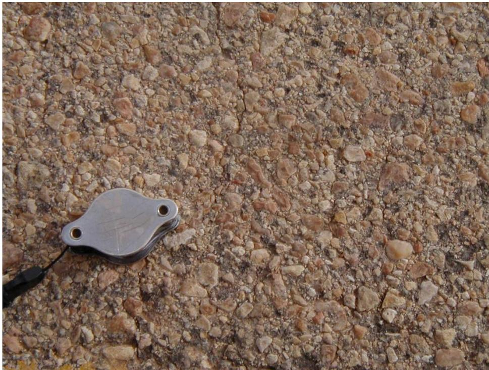
**Fig 14.** Crushed aggregate of carbonate rocks in the asphalt mixtures of Nalut-Ghadamis Road
