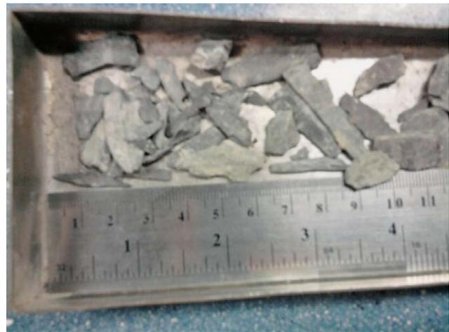
Figure 2: Rock particles cavings in shape of splinters (Zdravec, 2012)
