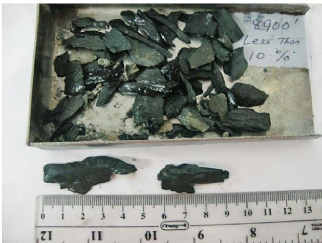
**Figure 4:** Rock particles cavings in shape of angulars (Zadravec, 2012)
