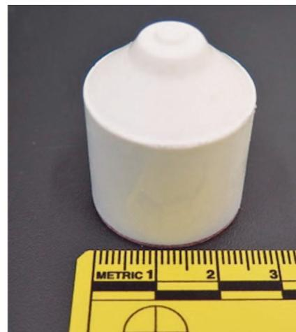
Figure 4: RDX Shaped Charge
