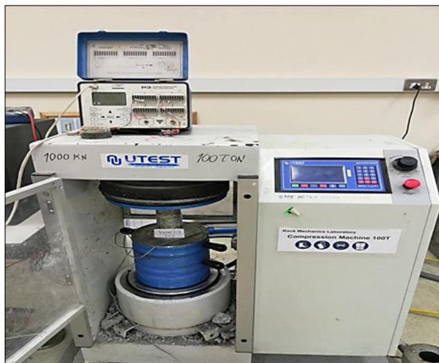
Figure 1. Uniaxial compressive testing machine
