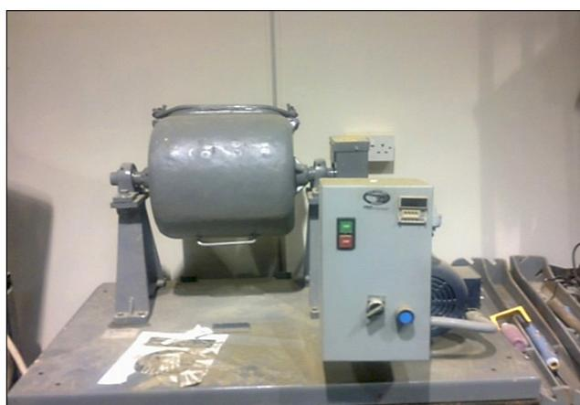
**Figure 8.** Lab ball mill
