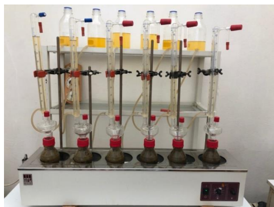
Figure 1. Laboratory reactor system for anaerobic digestion
