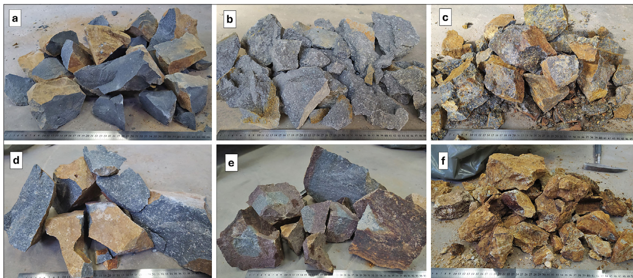
Figure 2. Photographs of the analysed rock samples. Samples labelled with “T” originate from the Tállya quarry, while those marked “R” are from the Recsk quarry. (a – T 1 ; b – T 2 ; c – T 3 ; d – R 1 ; e – R 3 ; f – R 4 ).
