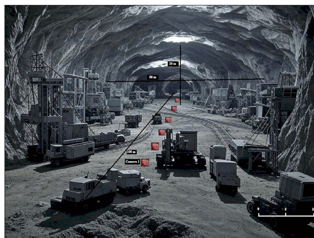
Figure 1. Synthetic underground mine model used for photogrammetric simulation. The 100 m × 50 m × 20 m tunnel network features irregular rock surfaces, mining equipment, and a diffuse lighting gradient (50 lux at center). Red dots indicate camera positions for image capture.
