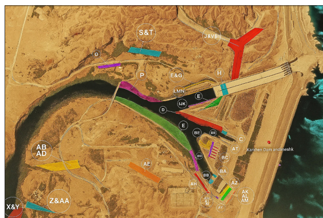
Figure 5: Location of the seepage measurement stations at the Karkheh Dam, monitoring discharge from the foundation and abutments.
